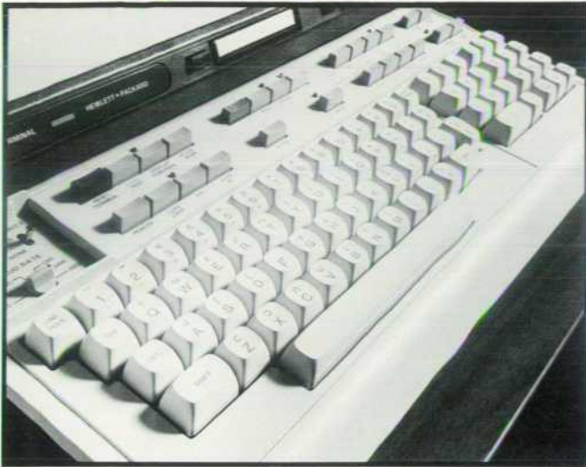
Fig. 4. 2641A keys have APL legends on top and ASCII legends, when they differ, on the front faces.
