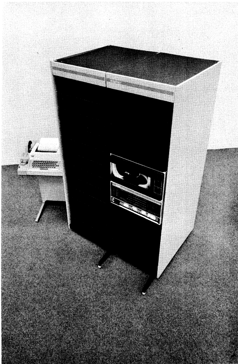
PDP-8/I—a full scale digital computer with an internal peripheral control and data break panel for plug-in expansion.
