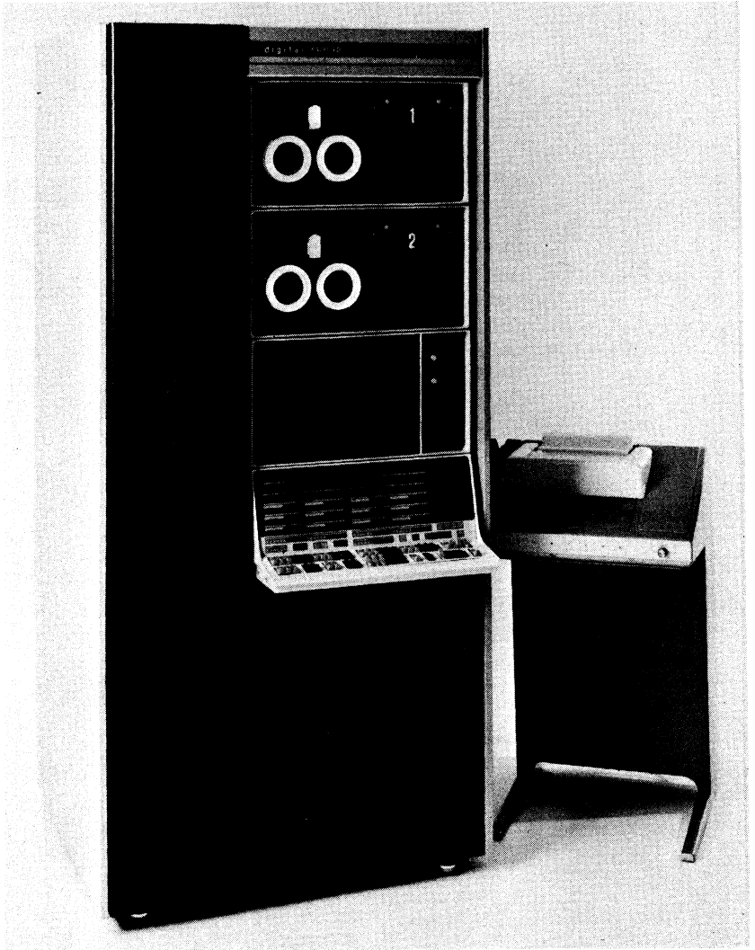
PDP-12—unified display-based programming system capable of executing LINC and PDP-8 family instructions.
